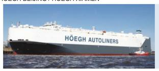
Vessel type: Pure Car and Truck Carrier (PCTC)
